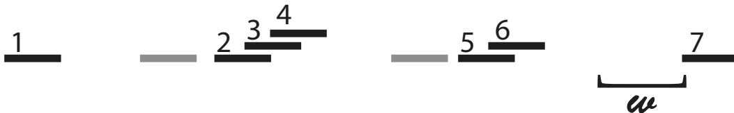
Figure 4: Interplay between tandem repeats and novel subset matches. There are two initial seed matches, one black, one gray. The black match has components labelled 1-7, and the neighborhood size w is shown with respect to component 7. As we attempt leftward extension of the black match we discover the gray match in the neighborhood of components 2 and 5 of black. A subset link is created. We also discover that some components of the black match are within each others' neighborhood. We classify the black match as a tandem repeat and construct a novel subset match with one component for each of the four tandem repeat units: \{1\} , \{2, 3, 4\} , \{5, 6\} , \{7\} .
